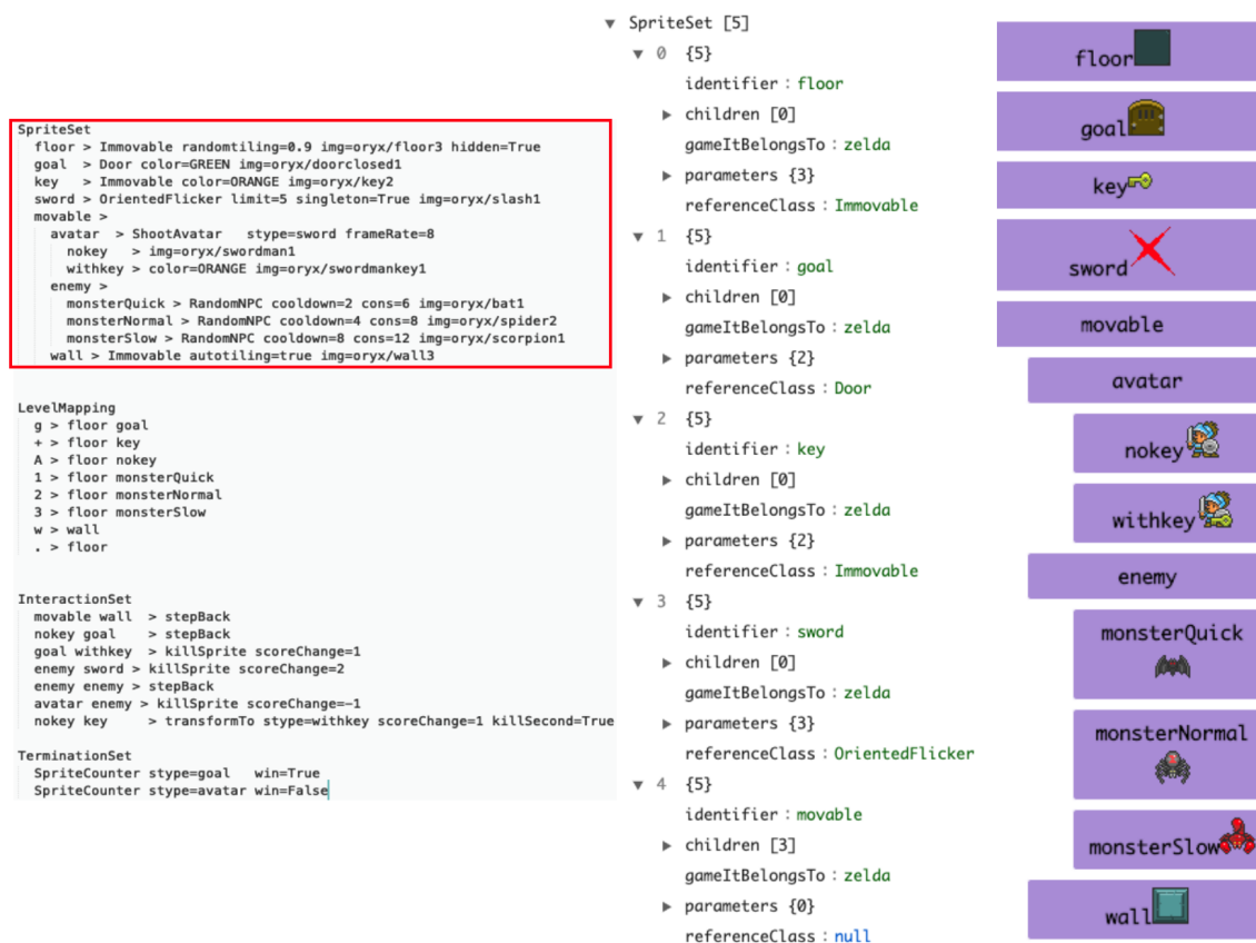
Figure 9.3: At the left side, the red square shows the SpriteSet of the VGDL version of the game Zelda. In the Center, it is exhibited a fragment of the SpriteSet converted to a JSON format. This format makes easier the process of navigating into the games and extract information from them. The referenceClass attribute that you can see in all the sprites listed in the JSON description (center figure) defines the behaviour of the sprite. At the right side you have a visualization of the whole SpriteSet . Every game in VGDL is converted to this format, and then, information are extracted, shared, and intertwined when the recommender system is applied to design games.
