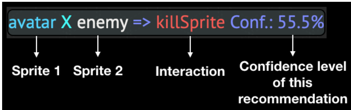
Figure 9.9: An example of an interaction recommendation component. The avatar sprite will be killed (killSprite interaction event) when colliding with a sprite enemy.
